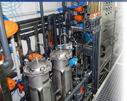
Treatment of leachate water from fermented communal wastewater sludge with forward osmosis (FO) and reverse osmosis (RO) technology.
