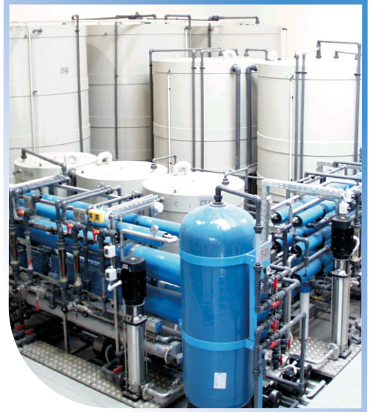
Purification and recycling of waste water from the manufacture of aircraft parts with ZLD technology. GE Aviation Hungary Ltd. / Magyarország 100 m 3 /day
